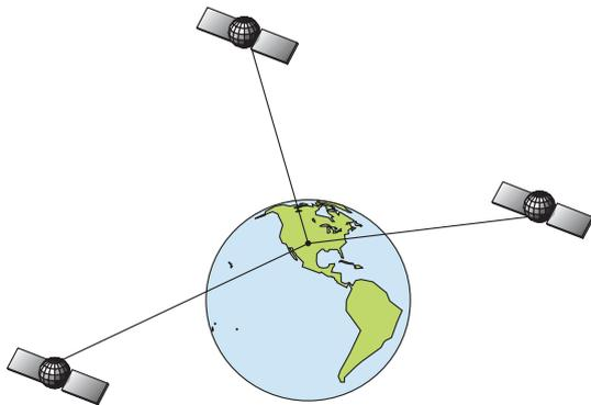
**A minimum of three satellites are required to determine a 2D fix.**
