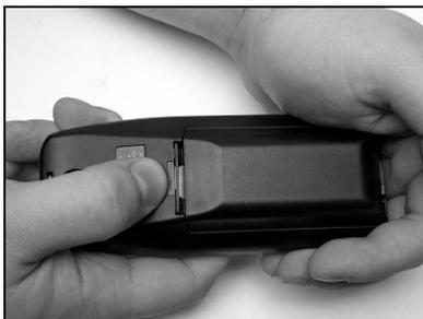
**Release the latch to remove iFINDER battery cover.**
