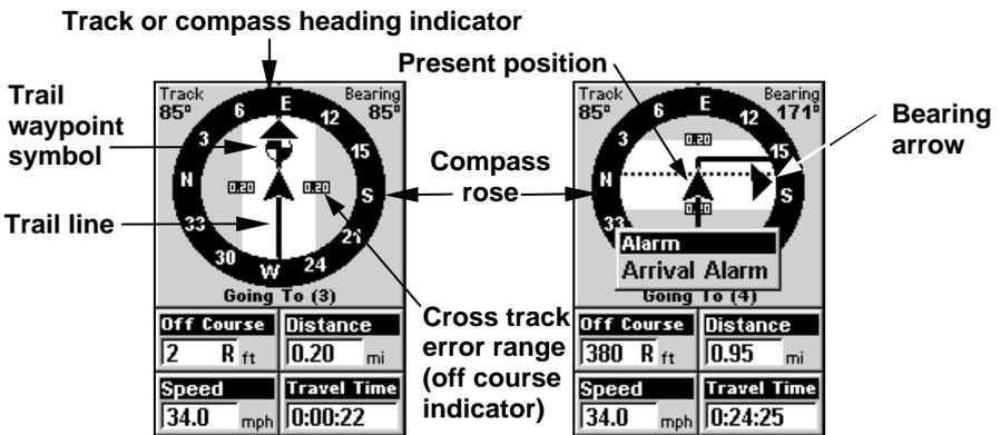
Navigate trail, navigation page (compass rose) views: at left, driver is eastbound heading straight toward trail point 3; bearing arrow shows the trail point is due east (straight ahead.) At right, driver has reached trail point 3 and must turn south to follow the trail. Arrival alarm goes off and bearing arrow swings around to say turn right (south), toward the next waypoint, trail point 4. iFINDER now shows navigation information to point 4, which is 0.95 miles away.
