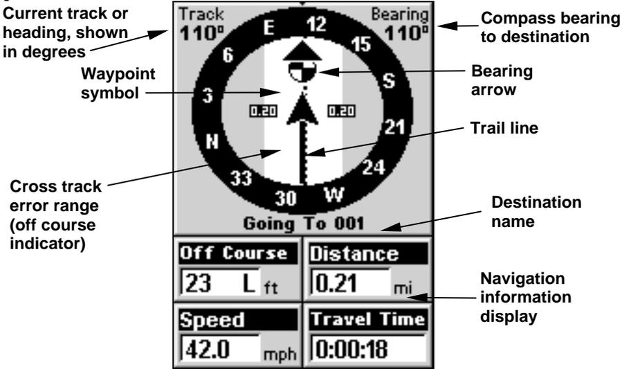
Navigation Page, backtracking a trail. Driver is headed due east (a 110° track) toward a waypoint 110° (bearing) away. The cross track error range (white corridor) is 0.20 miles either side of the course. The driver is headed toward waypoint 001, which is 0.21 miles away. The vehicle is very nearly on course (off course 23 feet). Traveling at a speed of 42 mph, the driver will arrive at the waypoint in 18 seconds.
